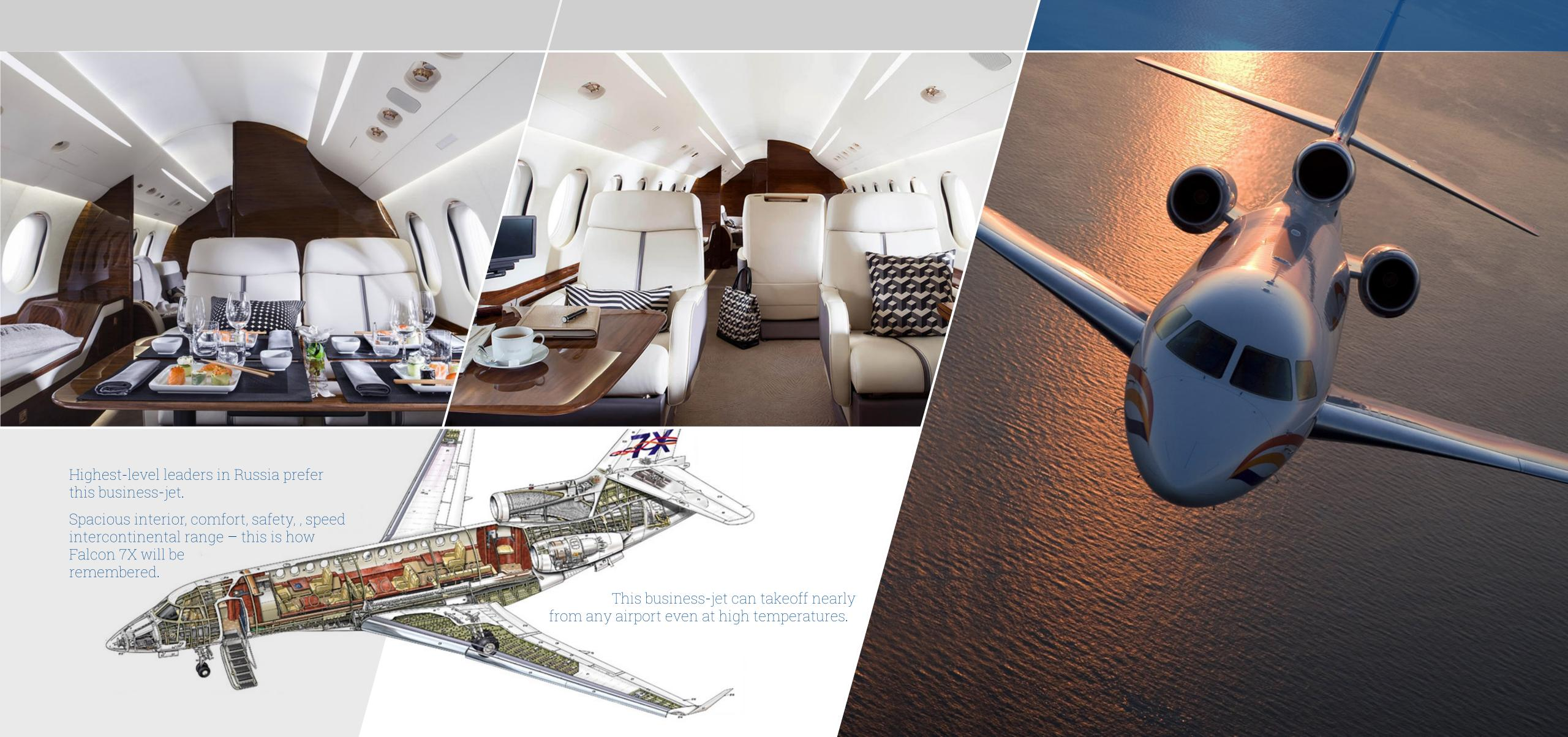
Specifications ensure a range of non-stop transcontinental flight. Cruise speed — 820 km/h, practical range – 5129 km, capacity — up to 14 passengers. 850
